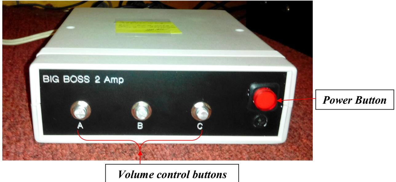
1. Press the **Red Button** to turn on/off the PA system.
